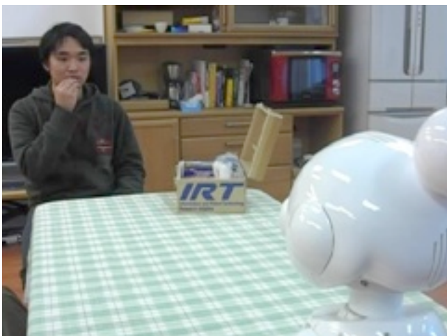
Mamoru watches the subject taking medicine. Visually recognizes and remembers when the subject brings the medicine box and prepares to take the medicine
