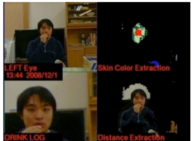
Visually recognizes when subject takes medicine Uses a combination of facial pattern recognition, focus on face and hands using 3-D recognition, and depth comparison
