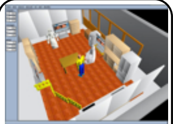
Recall support IRT technologies: Presentation viewer Positions of robot and user are recognized using SLAM and RFID
