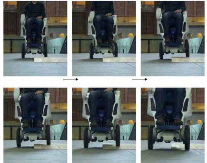
Fig. 4. Overcoming a slope of 50mm high
