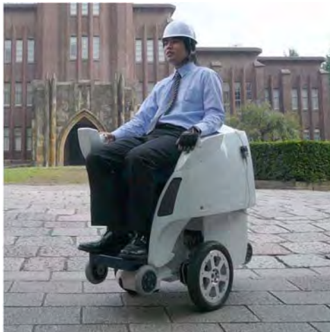
Fig. 3. The personal mobility robot
