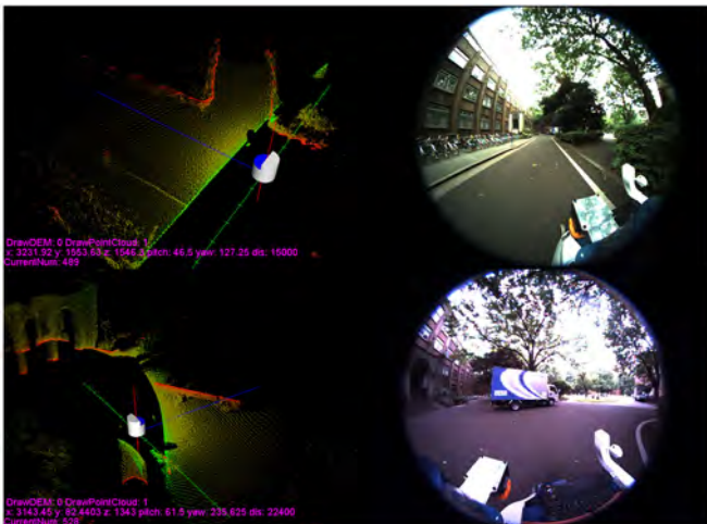
Fig. 7. Obstacle detection by a laser range finder outdoors
