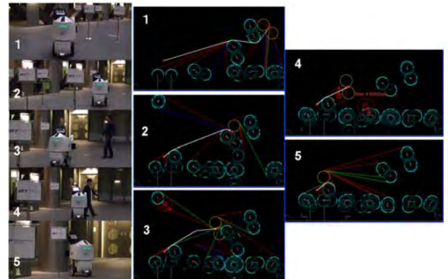
Fig. 12. Dynamic avoidance of collision and rerouting
